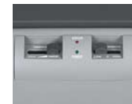
Left: continuously variable electronic thermostat; right: two-stage battery monitor
