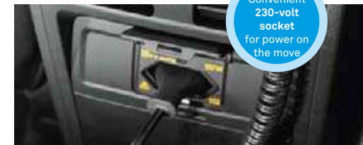
More and more European series-produced vehicle come with a 230-volt Euro socket. The required alternating voltage is generated by a WAECO inverter.
