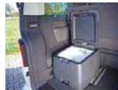
Thermoelectric cooler for the VW T5 Multivan, secured to the vehicle's floor rails with a customised fixing kit.
