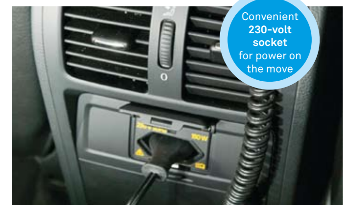
More and more European series-produced vehicle come with a 230-volt Euro socket. The required alternating voltage is generated by a WAECO inverter.
