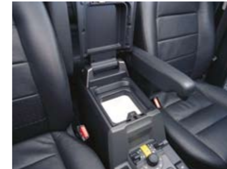
Dometic WAECO thermoelectric BordBar in the middle console: Land Rover Discovery 3 and Range Rover Sport
